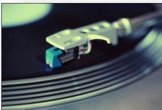
Although it isn't shown in the main picture, there will be a device below the head of the arm known as a cartridge and fitted into that will be a tiny stylus. It is the stylus that makes contact with the record, so it's important that it is clean and in good condition – don't touch it – they are delicate and expensive! It should look something like the one in the picture on the left.
